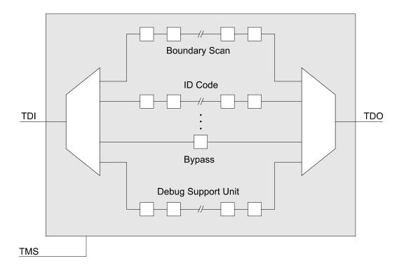
Figure 1: The data path through a single JTAG Test Access Port (TAP). The TAP Instruction Register (not shown) is a special scan register that selects which data scan register is connected between TDI and TDO.
