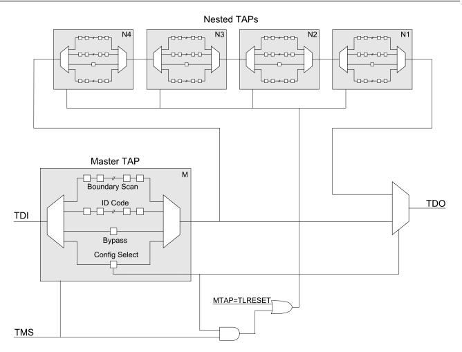
Figure 3: Nested TAP Architecture. The JTAG chain may be expanded to include all five TAPs, or collapsed to include only the master TAP, by setting the Config Select bit in the master TAP.
