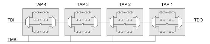
Figure 2: Four daisy chained JTAG TAPs. The TDO from each TAP is chained to TDI of the next to form one long scan chain. TMS is connected to all TAPs so that their state machines operate in unison, but because the instruction registers are concatenated, a different scan register may be selected in each TAP.
